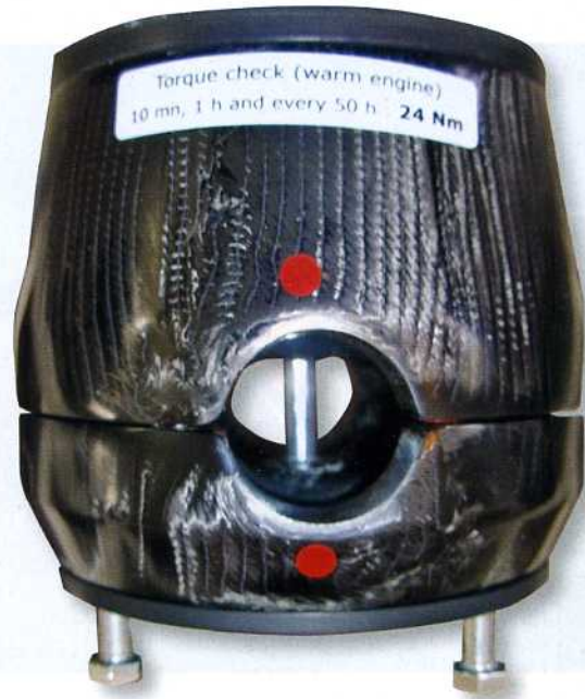
Left: Four blades on half of a prop hub, notice the color coding between the blades and the positions on the hubs.
